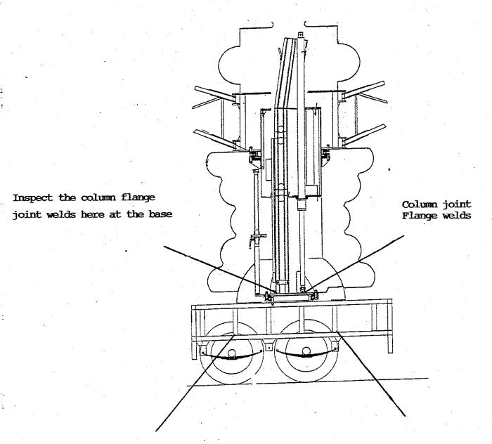
Inspect the lower frame welds here
