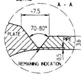
• GRNO GENTLY THE HARNESS PIPE IN ORDER TO OBTAIN TM BEVEL 'T' AS SHOWN IN VEW A-A TAKE CARE TO NOT 'PERFORATE' THE HARNESS PIPE (NOMINAL THICKNESS 36 mm)
