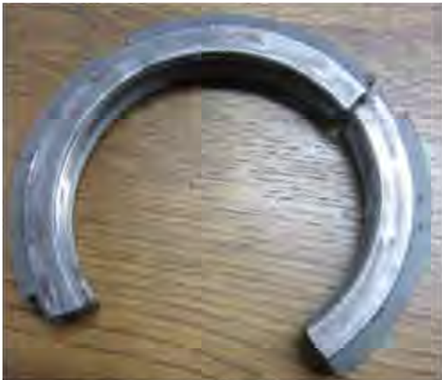
Figure 5: Broken KM nut due to use of improper tooling (assembly or disassembly)
