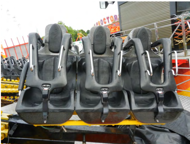
Figure 21 Alternate passenger restraint design
