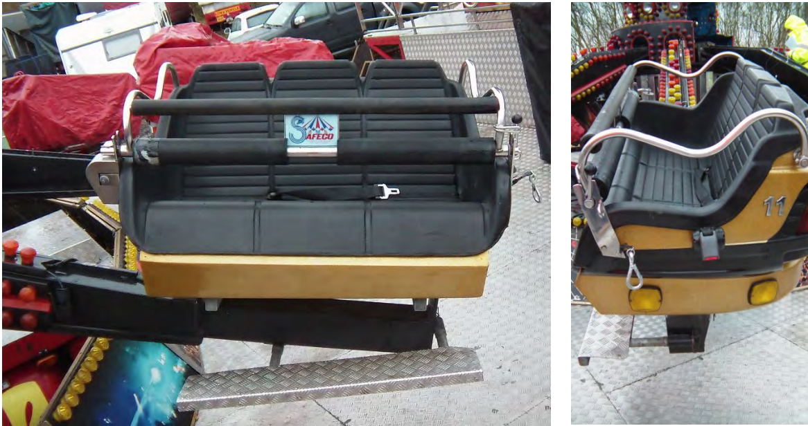
Figure 20 DJ Jump seating and restraint system
