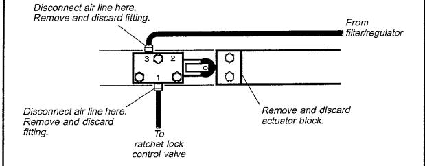
IMPORTANT: Do not disconnect both ends of these two lines; only disconnect them at the step interlock valve. Pay attention to where the lines are connected and how they are routed before disconnecting.
