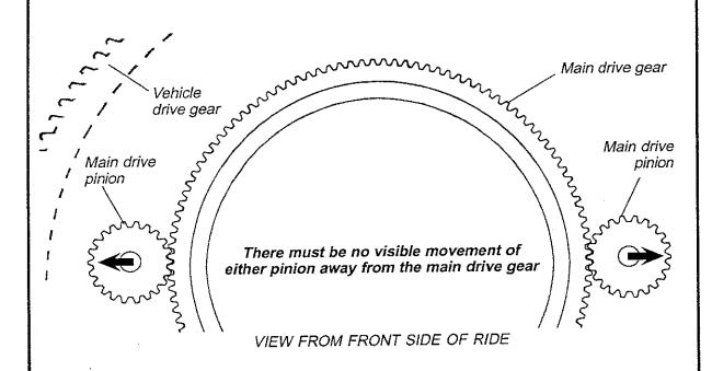
3. DAILY - Inspect both main drive gearboxes and all four vehicle drive gearboxes. If any gearbox exhibits oil leakage or excessively noisy operation, it is likely that failure of that gearbox has occurred
