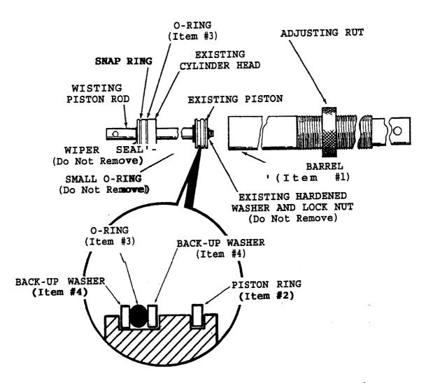
4. Install one O-ring (Item #3) on the existing cylinder head.
