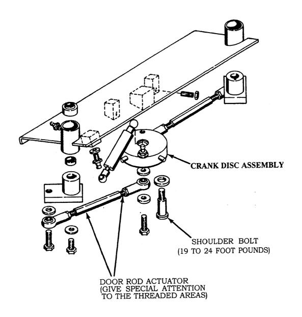
NOTE: If shoulder bolt holding the crank disc assembly is loose, remove, clean and reinstall using red Locktite and 19 to 24 foot pounds of torque.
