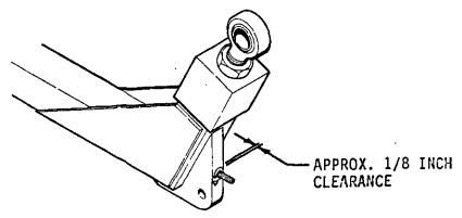
5. Install the reworked spreader bar. Repeat the procedure for all remaining long spreader bars.
