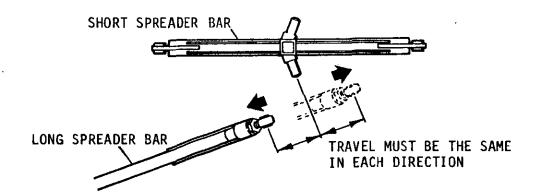
7. If the travel is equal in both directions, install the spreader bar and tighten all jam nuts and set screws.
