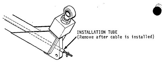
4. Remove the installation tube. Pull the cable tight by hand and install a cable clamp to allow approximately 1/8 inch clearance to the spreader bar.
