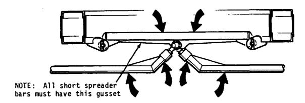
IMPORTANT: Do not attempt to repair spreader bars in the field. Any spreader bar which has been welded, drilled or otherwise repaired must be discarded and replaced with a new part.
