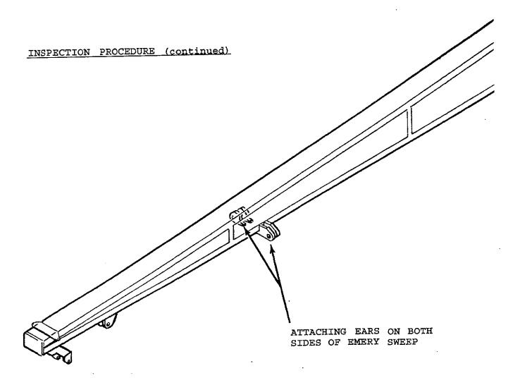
If your ride does not have a spreader bar attaching ear on both sides of every sweep, you must install the remaining ears before replacing the spreader bar system. Order the following kit:
