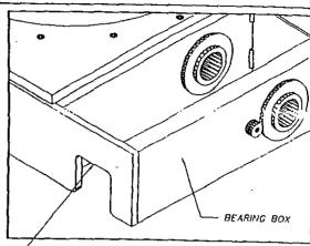
NOTE: INSPECT TOP AND SIDES OF THE MAIN LIFTING ARM AS THEY PASS THROUGH THIS OPENING FOR WEAR AND CRACKS ON BOTH ARMS.
