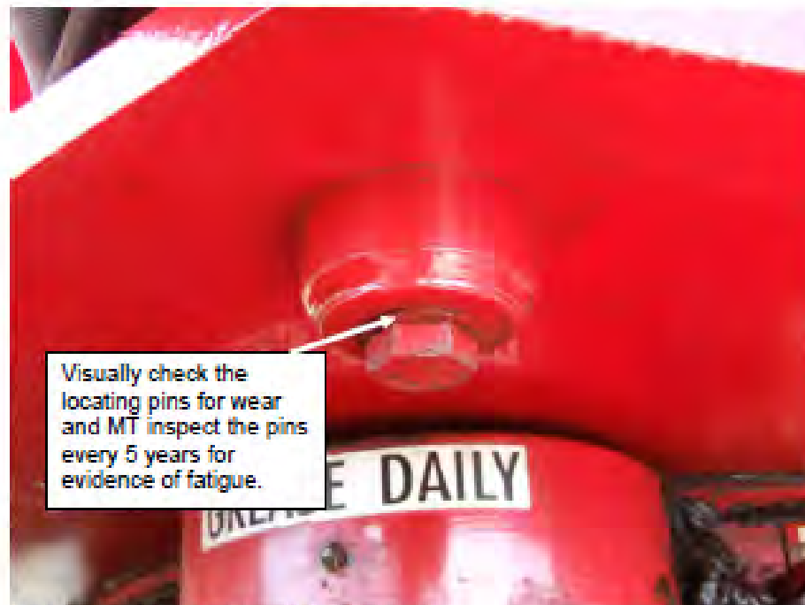
Fig 9: Retaining pins that prevent the arms folding.
