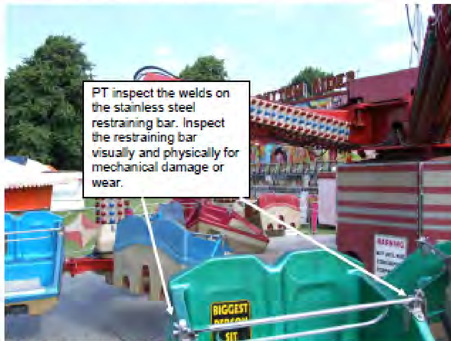
Fig 13: Passenger restraint bars fabricated from stainless steel.
