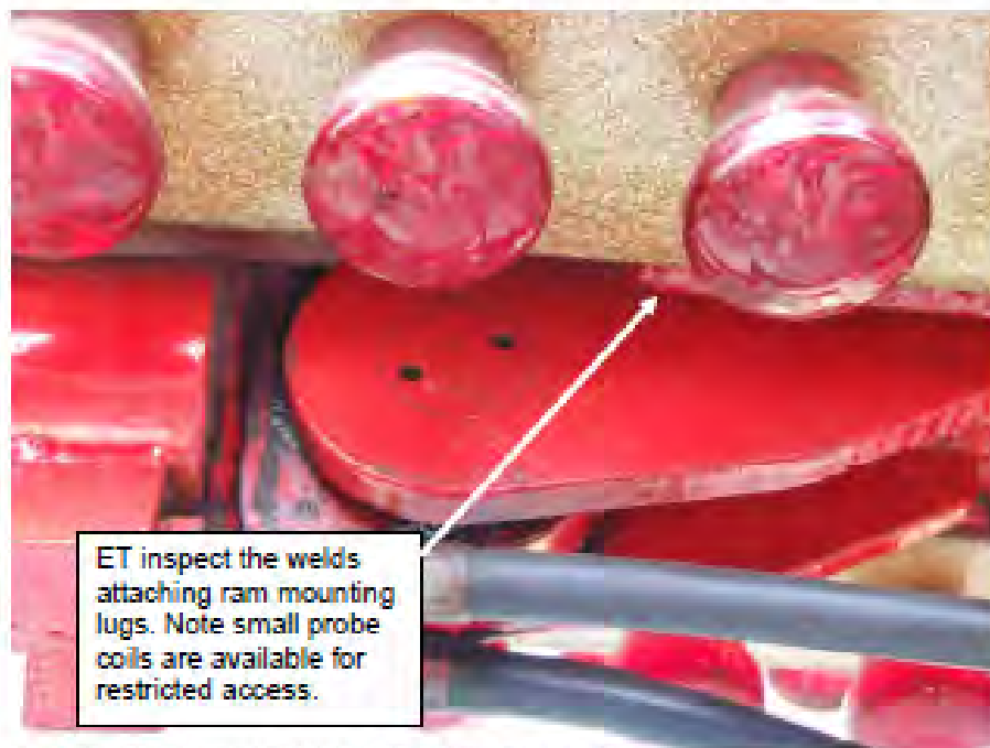
Fig 6: Attachment welds retaining the hydraulic ram on the arms.
