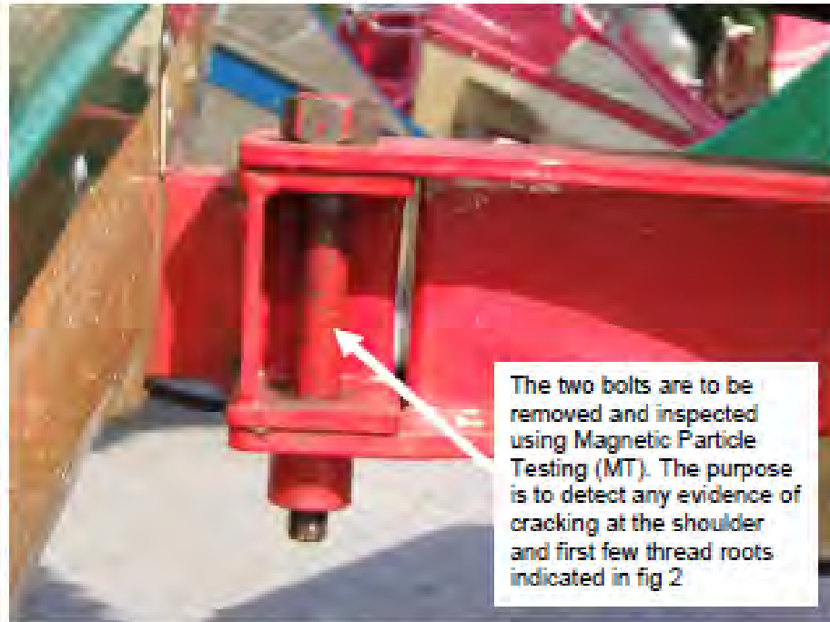
Fig 1: General view of the seat retaining bolt in position on the ride.
