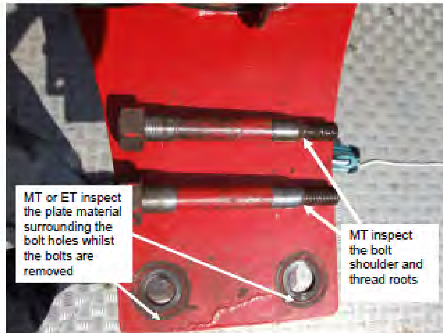
Fig 2: View looking down on the seat attachment arm with the seat assembly removed.
