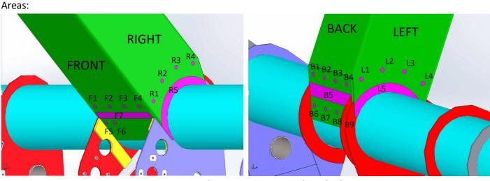
Spots L1, L2, L3, L4: Spots R1, R2, R3, R4: Spots F1, F2, F3, F4, F5, F6: Spots B1, B2, B3, B4, B6, B7, B8, B9: Areas L5, R5, B5, F7: Take measurement on described position. Test complete area and take smallest measurement over area.
