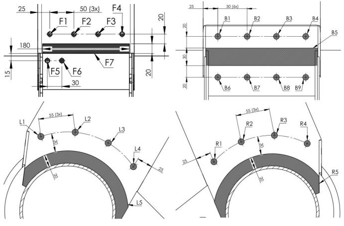
Accepted: All measured area meet a wall thickness >= 3mm.
