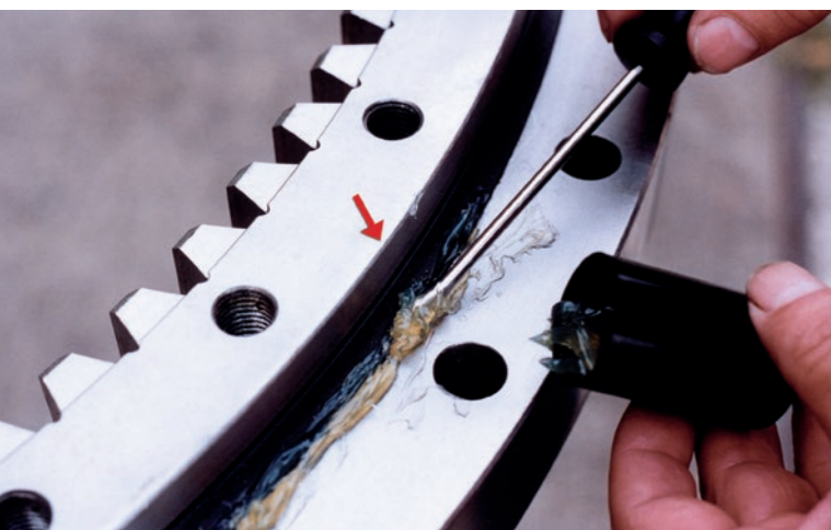
Figure 17: Taking a sample of grease from the sealing lip
